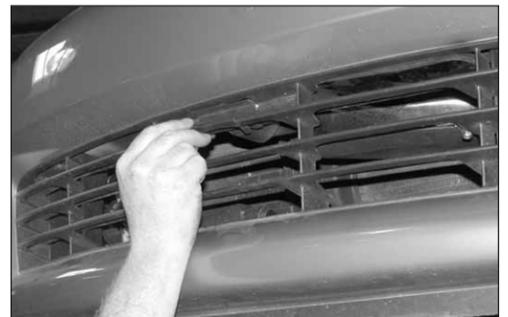
30. Reinstall the plastic grille insert as shown.
