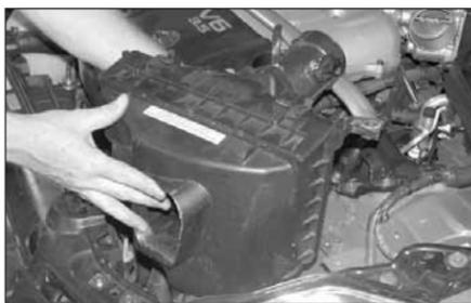
8. Pull the air cleaner assembly upwards then unclip the mass air sensor wire harness to remove the complete assembly.
