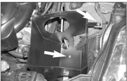
19. Reinstall the air box and secure it using the provided hardware as shown.
