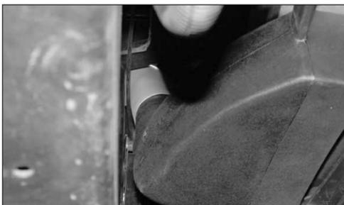
27. Slide the air inlet duct into the air inlet tube as shown, then, line up the bracket on the duct with the grille as shown.
