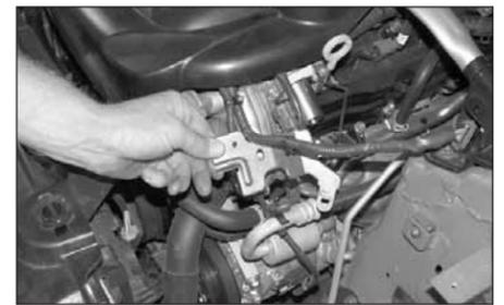
11. Remove the bolt that secures the mass air sensor harness bracket to the engine, then, remove the bracket as shown.
