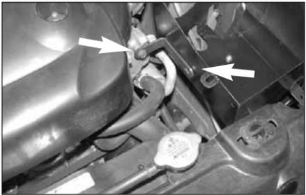
20. Using the bolt removed in step 11, secure the provided "L" bracket to the timing chain cover, then, secure the long leg of the bracket to the airbox using the provided hardware as shown.
