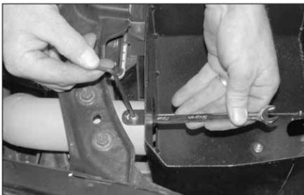
40. Tighten the hardware on the air inlet tube as shown.
