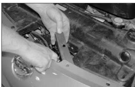
9. Loosen and remove the hex bolt that secures the Bumper cover bracket to the core support, then remove the bracket as shown.
