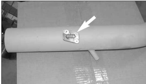
35. Install the mass air sensor into the Typhoon intake tube and secure with the provided hardware. **NOTE: Before installing the mass air sensor, inspect the inside of the tube for any debris, then clean the inside out with water and a towel. Inspect the tube one more time before proceeding to the next step.**
