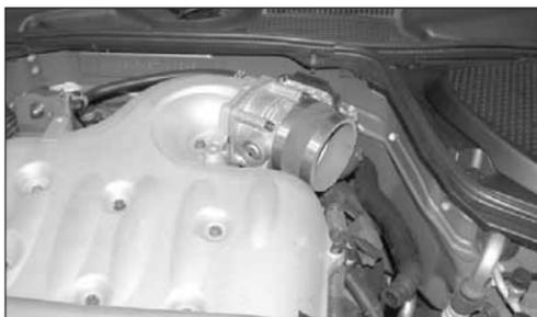
36. Install the silicone hose and hose clamps onto the throttle body as shown.
