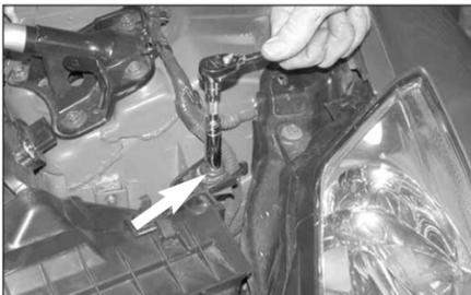
5. Loosen and remove the one bolt that secures the air cleaner to the inner fender hanger as shown.
