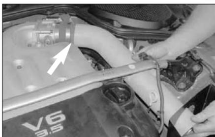
38. Slide the tube into the silicone hose on the throttle body as shown.
