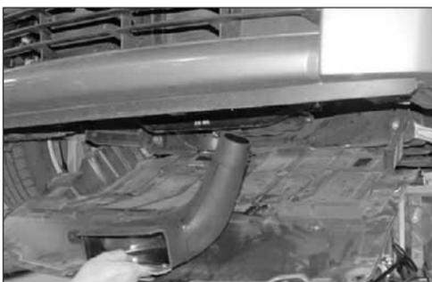
26. Install the air inlet duct from underneath the vehicle as shown.
