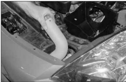
22. Slide the air inlet tube into the vehicle as shown. **NOTE: Before installing the intake tube, inspect the inside of the tube for any debris, then clean the inside out with water and a towel. Inspect the tube one more time before proceeding to the next step.**
