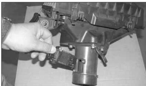
34. Remove the mass air sensor from the stock air cleaner assembly as shown.
