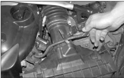
2. Unclip the wire harness from the air cleaner, then, disconnect the mass air sensor electrical connection as shown.
