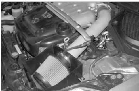
41. Install the K&N Air filter as shown.
