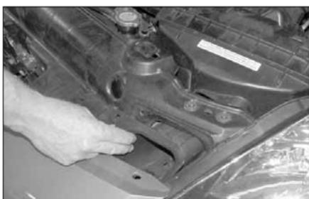
7. Pull the air inlet duct forward as shown.
