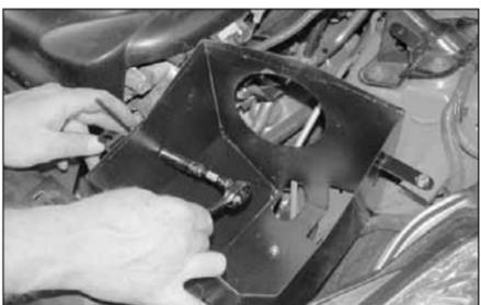
21. Adjust the air box for best fit and clearance, then tighten all the hardware on the air box as shown.
