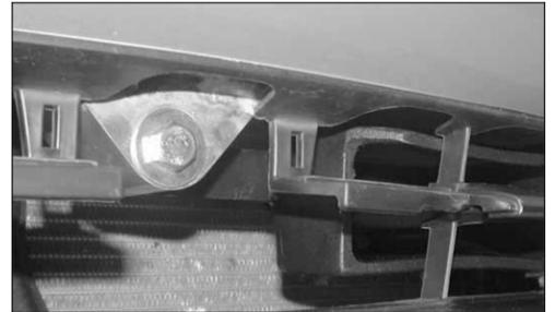
28. For 2003-2004, slide the shorter provided hex bolt through the aluminum cross member and slide the provided washer onto the hex bolt as shown. For the 2005-2006 model, slide the longer hex bolt and washers through the aluminum cross member.
