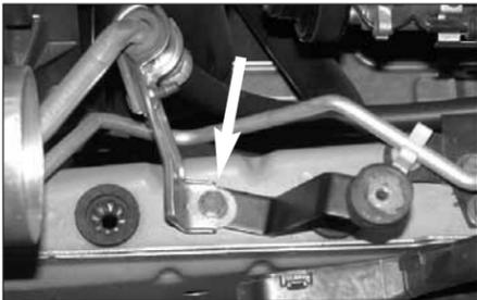
16. Using the bolt removed in step 14 secure the "Z" bracket underneath the air conditioner hardline bracket to the threaded hole from step 14. Do not tighten completely.
