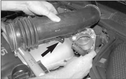
4. Loosen the hose clamps at the throttle body and at the mass air sensor, then, lift up the intake tube to disconnect the crank case vent hose, then remove the intake tube from the vehicle.
