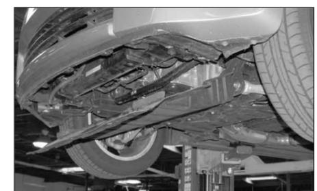
13. Remove the 12 hex bolts and 1 plastic rivet, then, lower the splash guard as shown.
