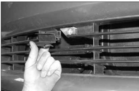
25. Remove the plastic grille insert from the vehicle as shown.
