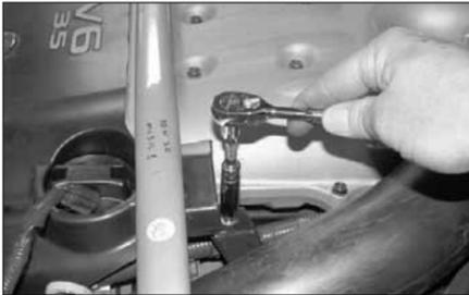
3. Loosen and remove the bolt that secures the intake tube to the intake manifold as shown.
