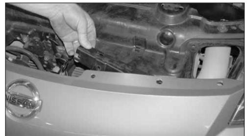
32. Reinstall the bumper cover bracket as shown and secure it with the stock hex bolt from step 9.
