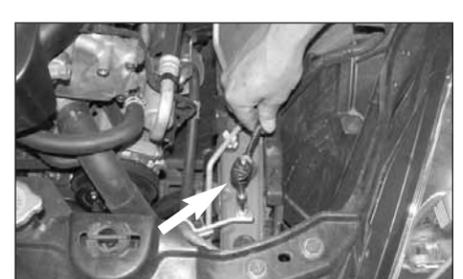
14. Remove the bolt that secures the air conditioner hard line bracket to the inner fender as shown.
