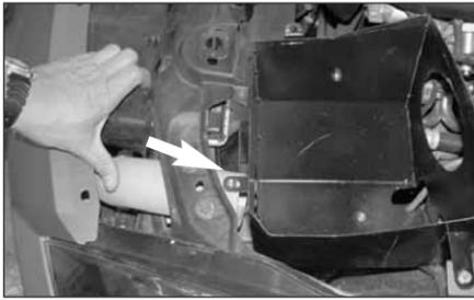
23. Secure the tube to the tab on the air box using the provided hardware but do not tighten at this time.
