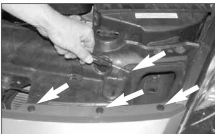
6. Remove the three plastic rivets from the bumper cover and the one plastic rivet from the air inlet duct as shown.
