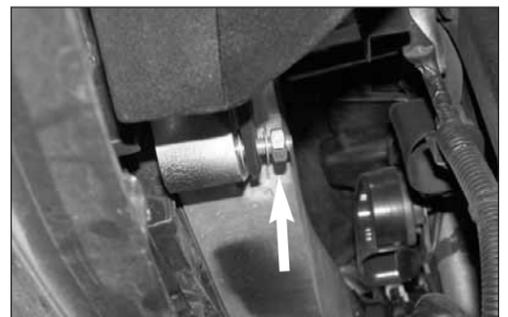
29. Slide the molded duct bracket onto the bolt from step 28, then, slide another washer and hex nut onto the hex bolt and tighten as shown.
