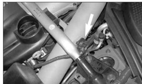
44. Reconnect the mass air sensor electrical connection as shown.
