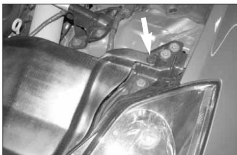
43. Secure the air box cover to the fender support bracket using the plastic rivet from step 6 as shown.
