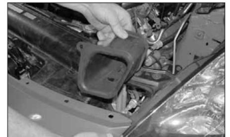
10. Pull the bumper cover forward and remove the air inlet duct as shown.
