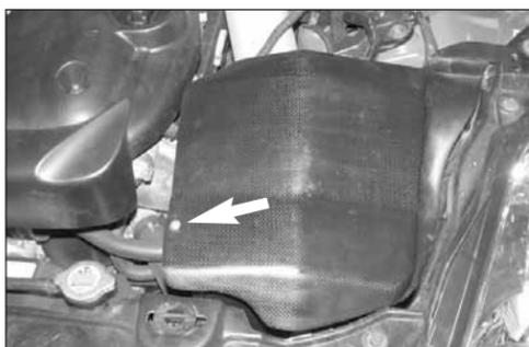
42. Install the air box cover and secure it with the provided hardware as shown.
