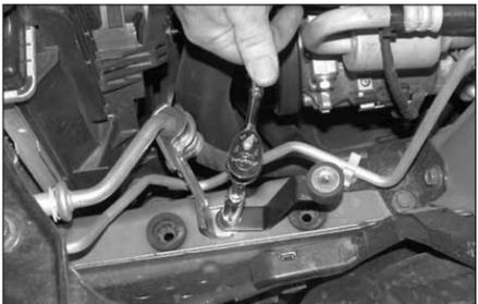
18. Remove the air box, then, tighten the "Z" bracket being careful not to move the bracket.
