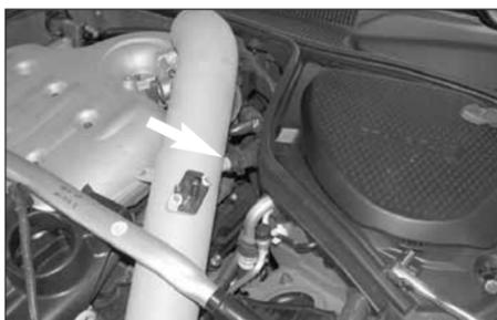
37. Slide the Typhoon tube into the engine compartment, then, reconnect the crank case vent hose to the vent on the K&N intake tube as shown.
