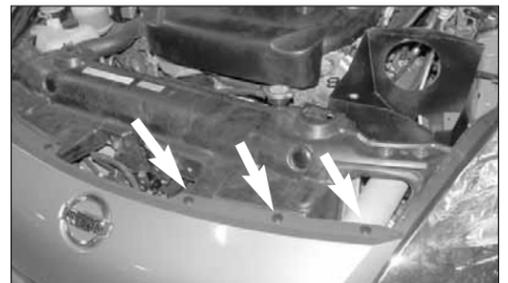
33. Reinstall the plastic rivets to the bumper cover as shown.
