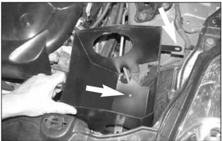
17. Install the K&N air box into the vehicle and line up the mounting tab with the original hanger, then line up the lower mounting hole with the rubber mounted stud from step 16.
