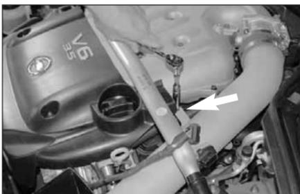
39. Secure the tube bracket to the intake manifold using the bolt removed in step 3.
