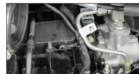
16. Unhook the wiring harness clip from the mounting stud, route the harness next to the coil and fuel line and secure the harness to the fuel line with the provided tie wrap.
