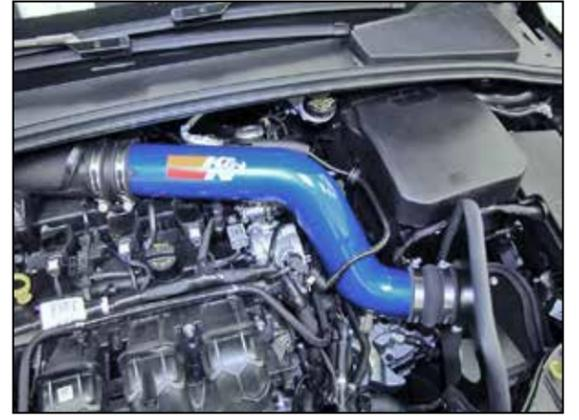
17. Install the K&N® intake tube into the factory coupler and then into the K&N® coupler, adjust the tube for best fit and then secure with the provided hose clamps.
