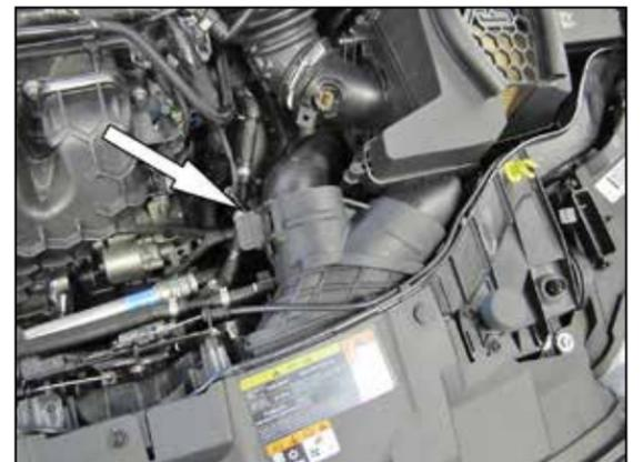
5. Release the inlet air duct from the air box.
