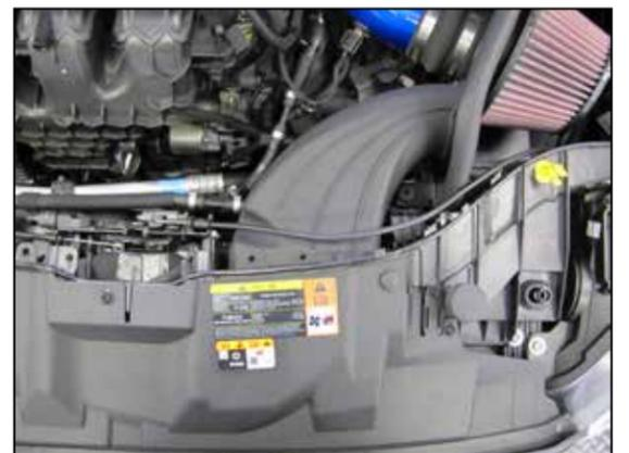
20. Install the K&N® fresh air duct onto the core support and into the K&N® heat shield.
