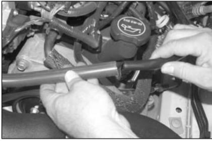
18. Using a razor blade cut the crank case vent tube 6" from the end as shown.
