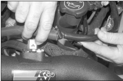
19. Install the provided crank case vent hose onto the K&N intake tube and factory vent hose as shown.
