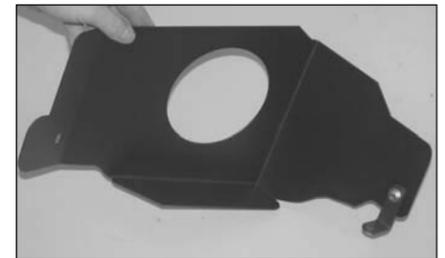
9. Install the "L" bracket (070812) onto the rear of the heat shield as shown with the provided hardware.
