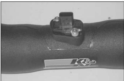
15. Install the mass air sensor into the K&N intake tube with the factory mounting screws and and two spacers provided.
