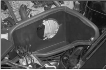
13. Install the heat shield and secure with the provided hardware as shown.
