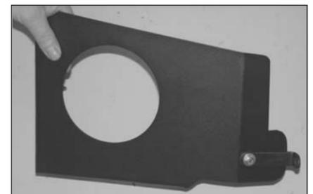
10. Install the "L" bracket (07158) onto the front of the heat shield as shown with the provided hardware.
