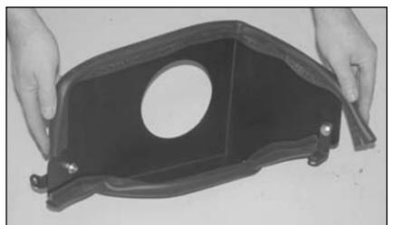
11. Install the edge trim onto the heat shield as shown.
