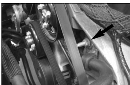
7. Remove the power steering pump bracket-retaining nut shown.
