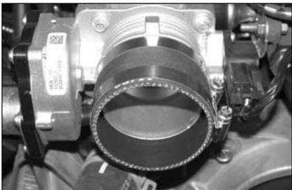
16. Install the silicone hose (08622) onto the throttle body with the provided hose clamps as shown.
