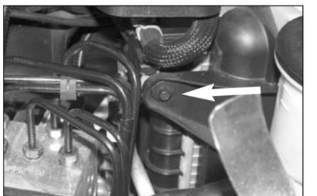
12. Remove the radiator fan shroud mounting bolt shown.
