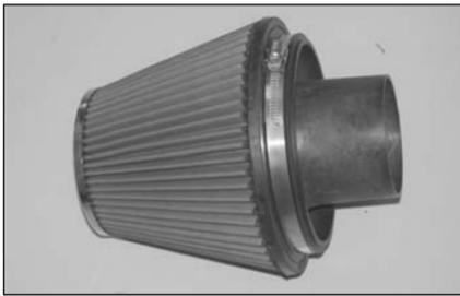
20. Install the FILTERCHARGER onto the filter adapter and secure with the provided hose clamp as shown.
