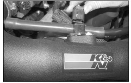
23. Reconnect the mass air sensor electrical connection as shown.
