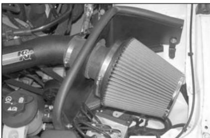
22. Install the FILTERCHARGER assembly onto the K&N intake tube as shown and secure with the provided hose clamp.
