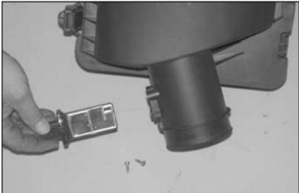
14. Remove the mass air sensor from the factory air box with the T20 "TORX" wrench provided.
