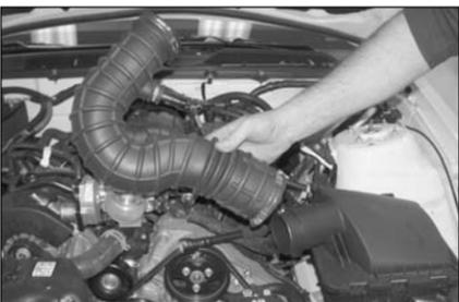
4. Loosen the hose clamps, which secure the intake tube to the throttle body and air box, then remove the intake tube as shown.
