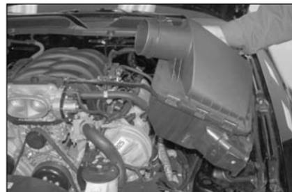
6. Remove the air box assembly as shown.
