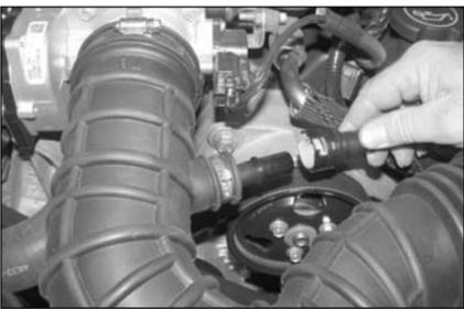
3. Release the red locking tab and then disconnect the mass air sensor electrical connection.
