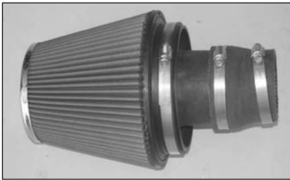
21. Install the silicone hose (08724) onto the Filtercharger assembly and secure with the provided hose clamp as shown.
