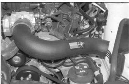
17. Install the K&N intake tube into the silicone hose at the throttle body and onto the tube-mounting bracket installed in step #8, secure with provided hardware.
