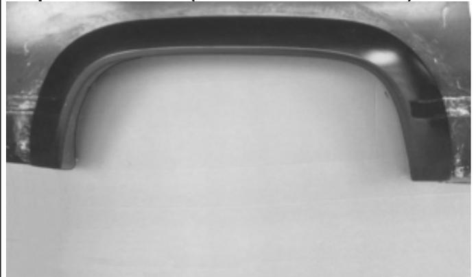
Place the flare on the vehicle. Apply 1 J-Clip into the mounting slots in the flare and secure it to the vehicle. Use 4 U-Clamps and secure it into the hole with hex screws as shown.
