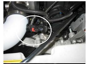
**p)** Reconnect the IAT sensor harness connector and secure.
