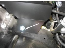
f) Secure the bottom of the heat shield with the fender washer and nylock nut.
