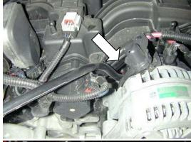
**o)** Check for clearance of the breather hose around the alternator and connector.
