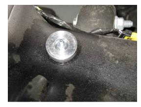
c) Secure the  $\frac{1}{4}$ -20 bolt and washer with the  $\frac{1}{4}$ -20 nut and tighten.
