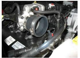
**h)** Attach the coupler to the throttle body and secure with #44 and #52 hose clamp.
