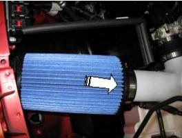
**q)** Attach the filter element and secure with #60 hose clamp.
