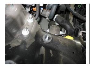
**b)** Insert the ¼-20 bolt and ¼" washer from underneath the grommet through the fender well.
