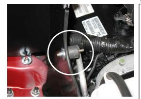
I) Install the rubber mount, fender washer and M6 nut onto the heat shield.
