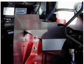
d) Insert the heat shield as shown. Align the heat shield to the studs in step 2g. The bottom of the heat shield should align with the stud from step 3c.
