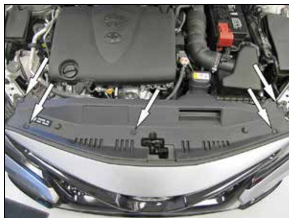
2. Remove the five push pins that secure the radiator cover and then remove the radiator cover.
