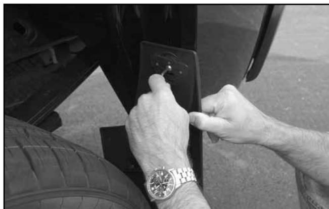
**8** While continuing to hold the MudFlap in place, tighten the upper QuickTurn™ fastener. The indicator (on the fastener) will again rotate 90° to the locked position. Continue rotating the hex head bolt until the MudFlap is tightly clamped to the fender lip.
