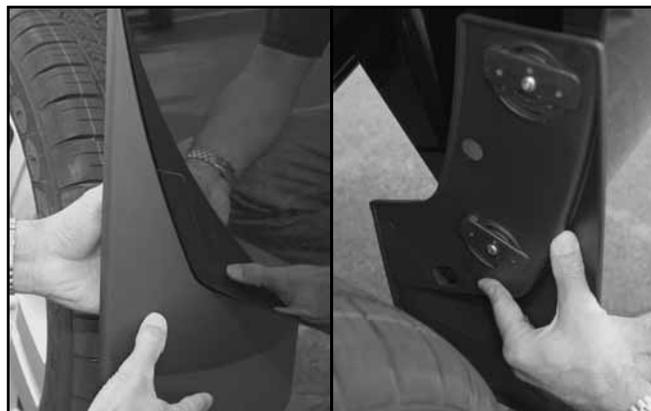
**6** When the lip edge has been hooked, rotate the MudFlap up into position onto the edge of the fender. The MudFlap will fit perfectly to the contour of the fender.
