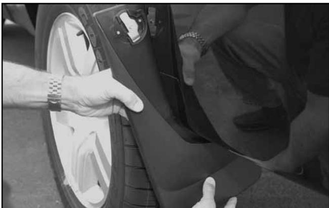
**5** While holding the MudFlap at approximately 45° from vertical (shown), hook the plastic tab on the MudFlap around the inside corner of the fender lip.
