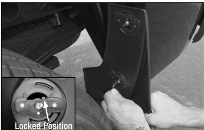
**7** While holding the MudFlap in place, use the hex key provided to tighten the lower QuickTurn™ fastener. The indicator (on the fastener) will rotate 90° to the locked position (indicated by padlock), continue rotating the hex head bolt until the MudFlap is tightly clamped to the fender lip (the bolt will have some resistance to turning).
