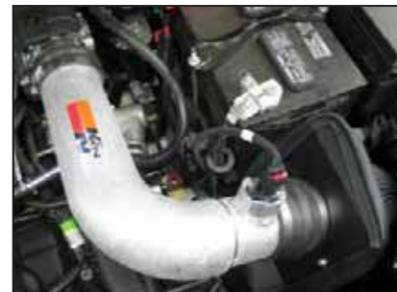
24. Connect the provided mass air sensor extension harness to the factory harness and connect the open end to the mass air sensor. Secure the mass air sensor extension harness to the vehicle wiring harness with the provided tie wrap.
