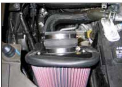
14. Install the silicone hump hose (5-576) onto the filter adapter and secure with the provided hose clamp.
