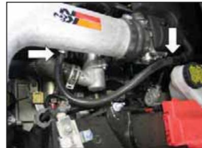
23. Connect the provided EVAP vent line to the fitting on the K&N® intake tube and then connect the open end to the factory EVAP check valve.
