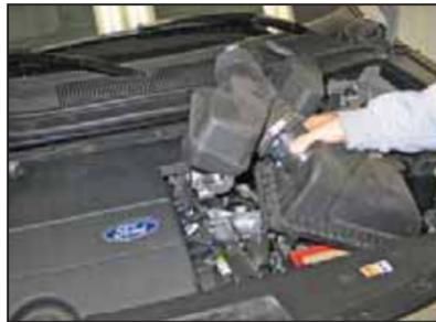
5. Release the two upper air box retaining clips and then remove the upper air box and intake tube assembly from the vehicle.
