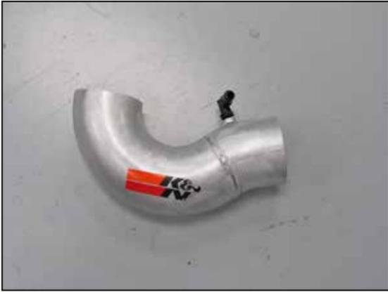
23. Install the provided 90° fitting into the K&N® intake tube as shown.
