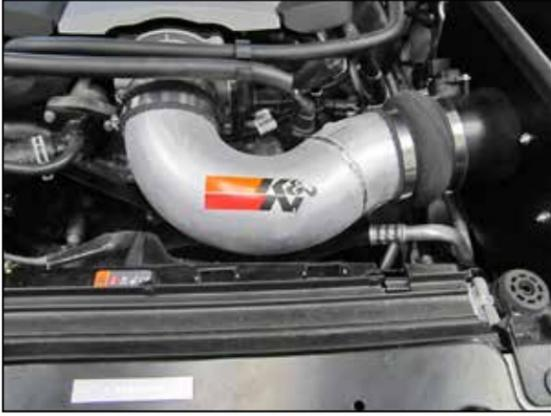
24. Install the K&N® intake tube into the hump coupler and then into the coupler at the throttle body, adjust the tube for best fit and then secure with the provided hose clamps.
