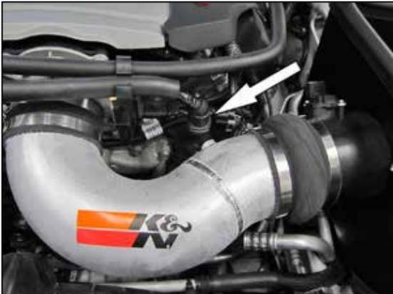
25. Connect the crank case vent hose to the quick disconnect fitting installed into the K&N® intake tube.
