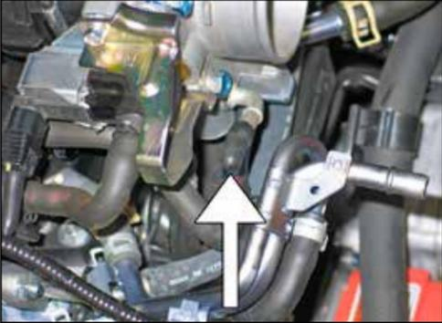
11. **Be sure the engine is cool before performing this step. Be sure to capture any released coolant.** Release the spring clamps securing the coolant bypass hose to the throttle body and the crankcase vent hose to the valve cover. Remove the bypass hose from the throttle body fitting, quickly plugging the outlet with a cap plug to prevent coolant loss. Remove the crankcase vent hose from the valve cover.
