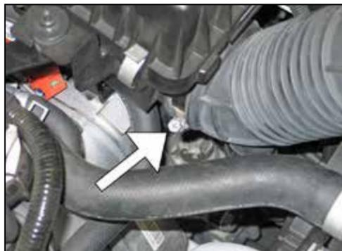
4. Loosen the hose clamp that secures the fresh air intake scoop to the airbox.
