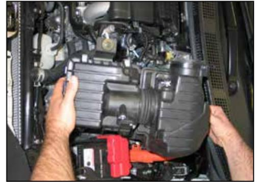
8. Remove the airbox assembly from the vehicle.
