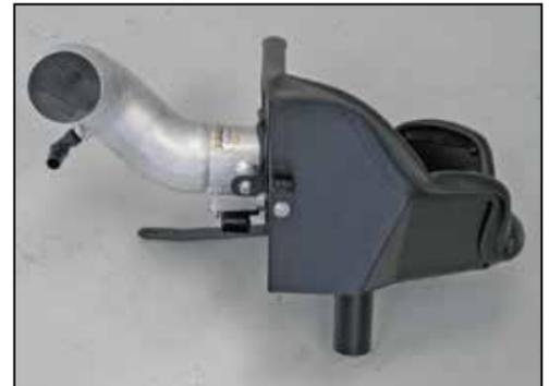
24. Install the K&N® intake tube into the heat shield and secure to the mounting bracket with the provided hardware.
