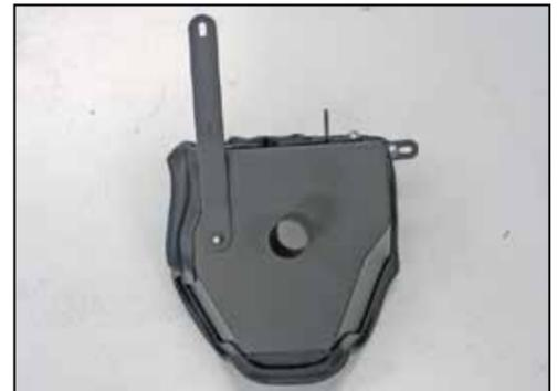
23. Install the flat bracket (083148) onto the heat shield as shown using the provided hardware.
