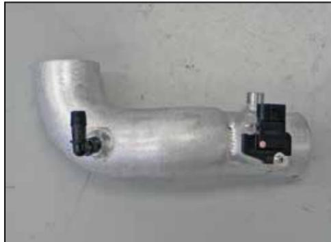
18. Install the provided 90° vent fitting into the K&N® intake tube as shown.
