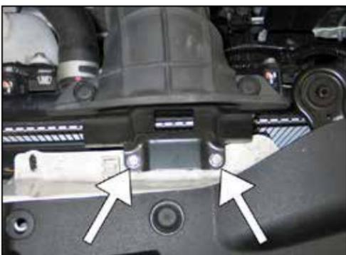
3. Remove the two bolts securing the fresh air intake scoop to the core support.
