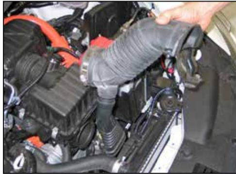
5. Remove the fresh air intake scoop from the vehicle.
