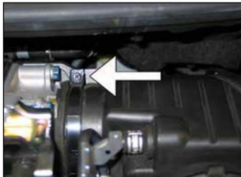
6. Loosen the hose clamp securing the intake hose to the throttle body.
