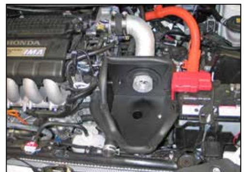
25. Install the heat shield/tube assembly into position and install the lower air duct onto the tube on the heat shield. Secure the heat shield to the factory airbox mounting locations with the hardware provided. Then secure the intake tube to the throttle body hose with the provided hose clamp.
