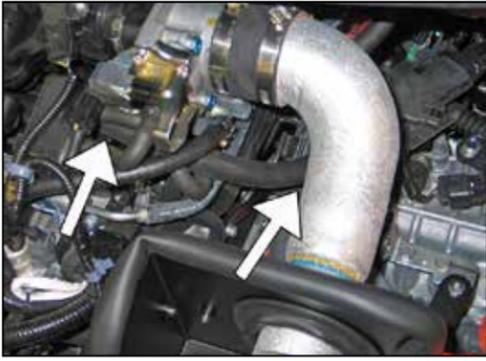
26. Attach the provided crankcase vent hose to the valve cover port, and then attach the open end to the 90° fitting in the intake tube.
