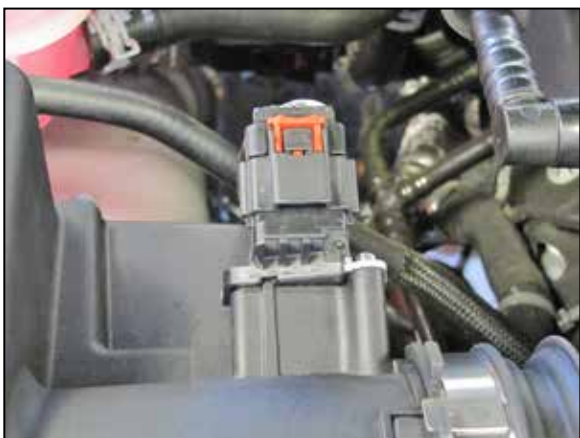
2. Disconnect the mass air sensor electrical connection.
