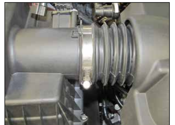
4. Loosen the hose clamp that secures the intake tube to the air filter housing.
