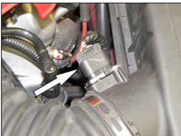
2. Disconnect the mass air sensor electrical connection.
