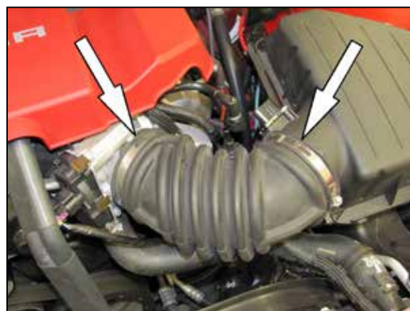
4. Loosen the two hose clamps securing the factory intake and then remove the factory intake hose.
