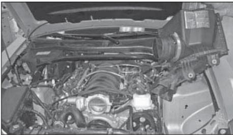
10. Remove the air box assembly from the vehicle.
