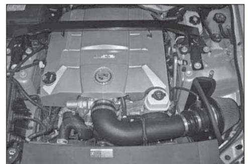
25. Reinstall the engine cover and radiator cover. Secure the radiator cover with the factory retainers.
