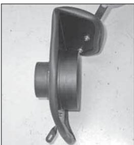
16. Assemble the mass air sensor and filter adapter with the provided gaskets onto the heat shield as shown using the provided hardware.
