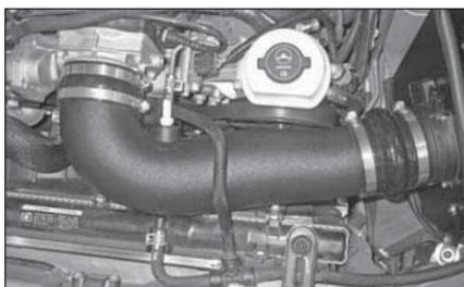
22. Install the K&N® intake tube onto the mass air sensor and then into the silicone hose on the throttle body. Secure the intake tube with the provided hose clamps.
