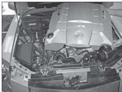
6. Lift up the engine cover to dislodge it from the mounting grommets and then remove the cover from the vehicle.
