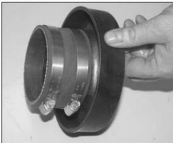
28. Install the provided silicone hose (#08698) onto the K&N filter adapter as shown.
