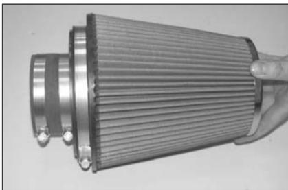
29. Install the filter adapter assembly into the K&N filter charger element.
