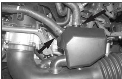
4. Remove the two vent lines from the air intake resonator as shown.
