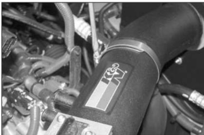
25. Secure the K&N intake tube to the saddle bracket with the provided hose clamps, also tighten the hose clamp at the throttle body.
