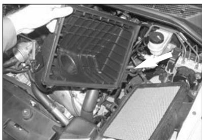
6. Release two airbox lid retainer clips that secure airbox lid to airbox, then remove airbox lid and air filter.
