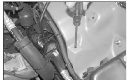
13. Using a screw driver, push the center of the plastic inner fender retaining clip through, then remove clip from inner fender.
