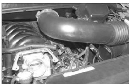
5. Loosen the hose clamps at the throttle body and airbox, then remove the intake tube from vehicle.
