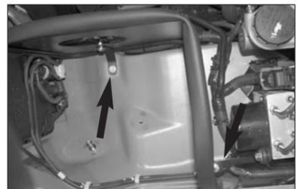
14. Install the heat shield onto the vehicle and secure with the provided hardware.
