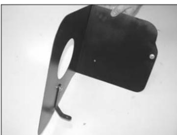
11. Install "L" bracket (07190) onto the K&N heat shield as shown.
