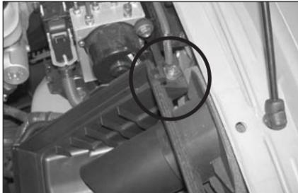
7. Remove the airbox mounting bolt with 10mm socket.
