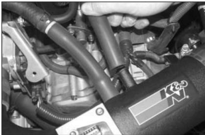
27. Install the provided silicone hose onto the hose mender, then install the hoses onto the K&N intake tube as shown.
