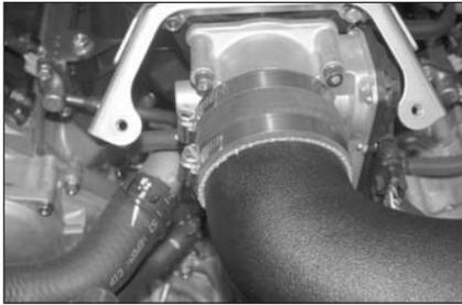
24. Install the K&N intake tube onto the throttle body and align with the saddle bracket.
