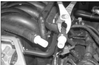
26. Install the provided hose mender into the two crank case vent hoses and secure the existing spring clamps as shown.
