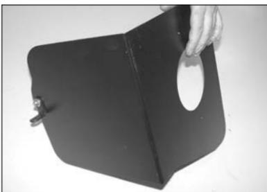
10. Install "L" bracket (#070066) onto the K&N heat shield as shown.
