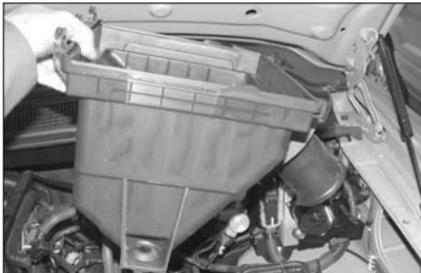
8. Pull firmly up on airbox to release from mounting studs, then remove airbox from vehicles.
