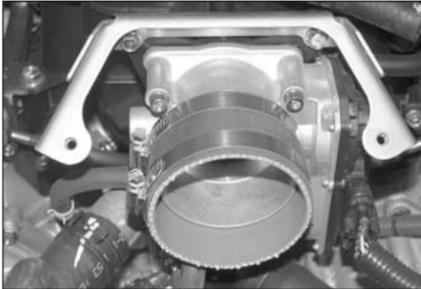
18. Install the provided silicone hose (08690) onto the throttle body with the provided hose clamps as shown.
