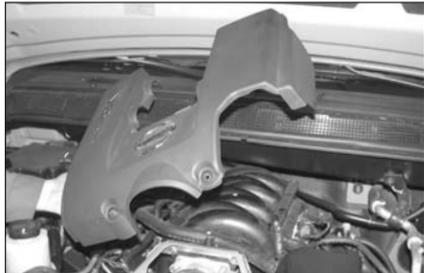
2. Remove the two bolts that secure the throttle body cover. Then remove the throttle body cover.
