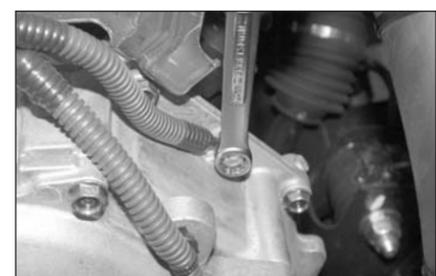
16. Remove ground wire attaching bolt on top of engine cam cover with 10mm wrench.
