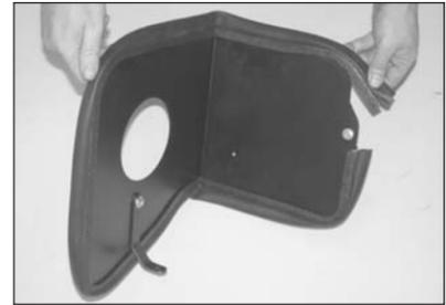
12. Install the edge trim onto the heat shield as shown. Trim as needed.
