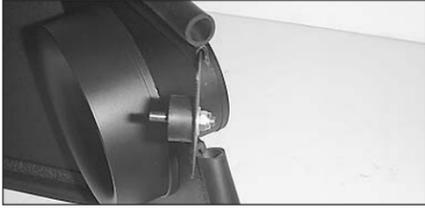
18. Attach a rubber mounted stud to the heat shield using the hardware provided. **Note: Do not tighten completely at this time.**
