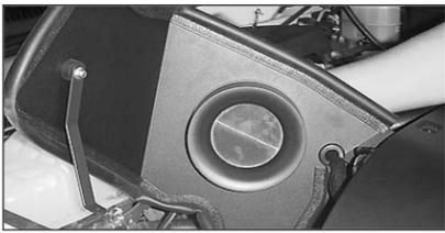
20. Install the heat shield assembly.
