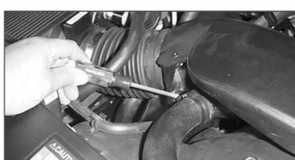
5. Using a flat blade screwdriver, pry the radiator hose retaining clip from the intake tube.
