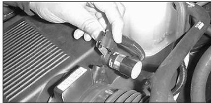
2. Disconnect the mass air sensor electrical connection.
