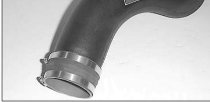
24. Install the 3.75"ID silicone hose onto the intake tube. **Note: Do not tighten the hose clamps at this time.**
