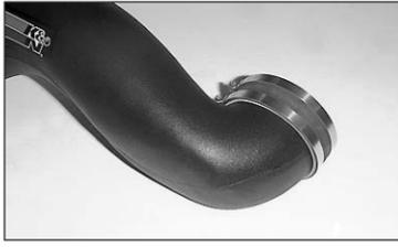
23. Install the 4"ID silicone hose onto the intake tube. **Note: Do not tighten the hose clamps at this time.**
