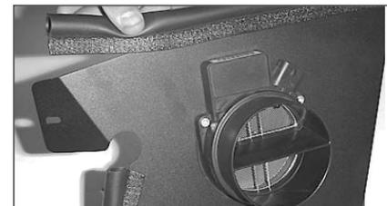
11. Install the trim seal onto the heat shield as shown.
