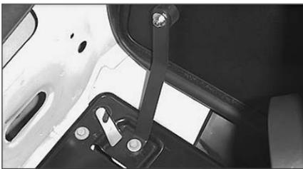
21. Secure the bracket to the airbox mounting tray using the bolt removed in step 19. **Note: Do not tighten completely at this time.**
