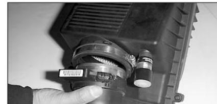
9. Loosen the hose clamp and remove the mass air sensor from the airbox.
