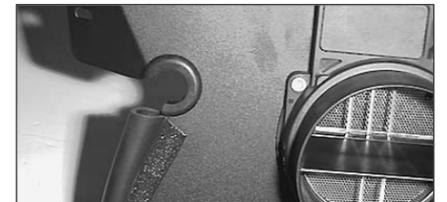
14. Install the grommet onto the heat shield.
