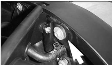
22. Secure the rubber mounted stud to the radiator mounting bracket.
