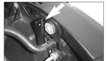
16. Measure over and down 1/2" on the radiator mounting bracket and mark.
