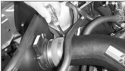
28. Tighten the hose clamp on the silicone hose at the intake tube.
