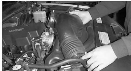
7. Detach the intake tube from the throttle body and remove the intake assembly.
