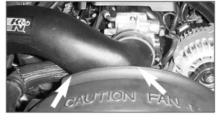
31. Due to production tolerances it may be necessary to mark the fan shroud as indicated, remove the intake tube and trim the fan shroud.
