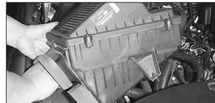
8. Pull firmly upward and remove the airbox.
