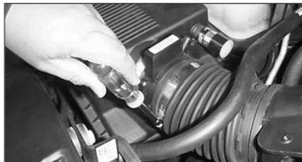
3. Loosen the hose clamp on the intake hose at the mass air sensor.
