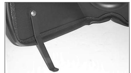
15. Attach the bracket assembly to the heat shield using the hardware provided.
