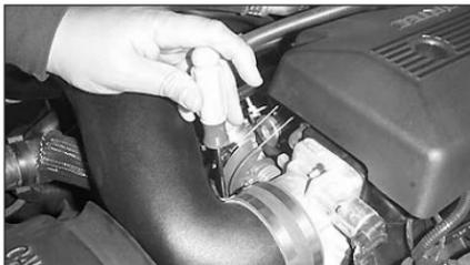
27. Align and check the intake tube for clearance, tighten the hose clamp on the silicone hose at the intake tube.
