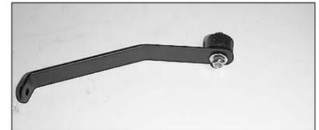
12. Attach the rubber mounted stud to the bracket.
