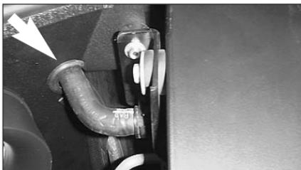
30) Insert the radiator over flow hose into the grommet on the heat shield.
