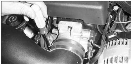
25. Install the intake tube and tighten the hose clamp on the silicone hose at the throttle body.
