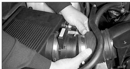
6. Detach the intake hose from the mass air sensor.
