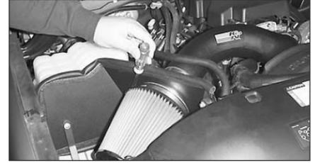
32. Install the Filtercharger element and secure with hose clamp.
