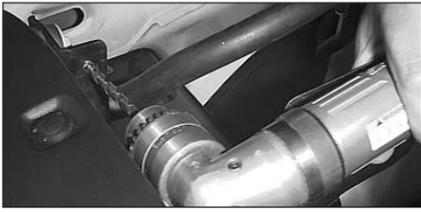
17. Using 1/4" drill bit, drill out location marked in the previous step.
