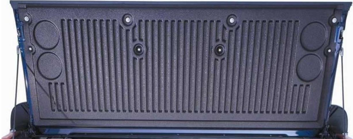
On the four outside bolts, place supplied metal washers on shoulder bolt and loosely attach panel. Return to the center bolts and retighten from center to outside bolts.
