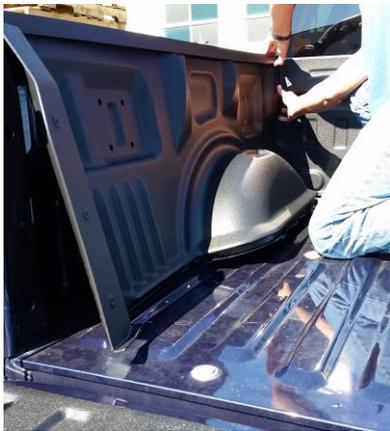
If your truck is equipped with LED lights, there are pre-cut holes for both lights and the switch. If your truck is equipped with a bed extender, you will see three pin marks at the back edge of the side panel that aligns with the holes for your bed extender. Open these up to the correct size with a drill bit and reinstall your bed extender.
