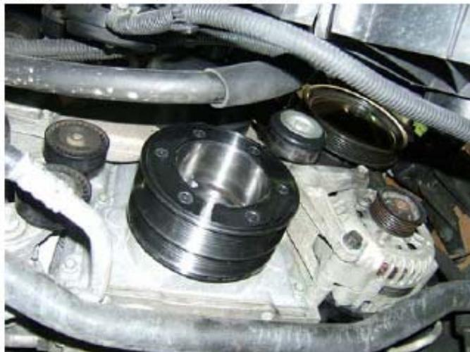
**Pic. 4** Crank pulley/balancer installed
