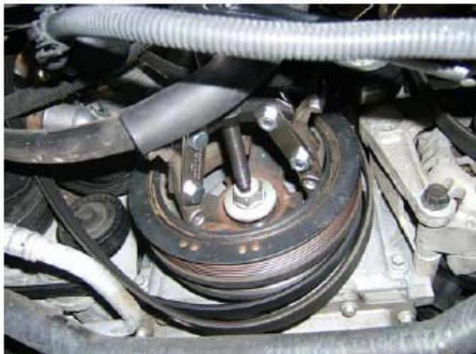
**Pic. 3** Using the puller tool
