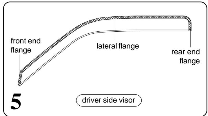
**STEP 6:** Align the driver side visor with the previously prepared rubber trim. Slide the front end flange under the mirror cap. Then, press the exposed areas of tape against the trim and verify position. See **FIGURE 6a**
