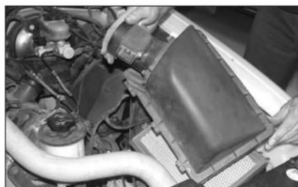
7. Release the 2 clips which retains the airbox lid then remove the lid from the vehicle.
