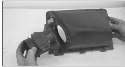
20. Remove the four bolts that retain the mass air sensor to the airbox lid, then remove the mass air sensor from lid.
