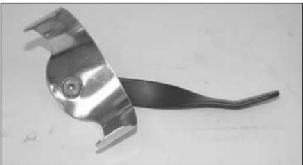
15. Using the provided hardware, assemble the saddle bracket assembly as shown.
