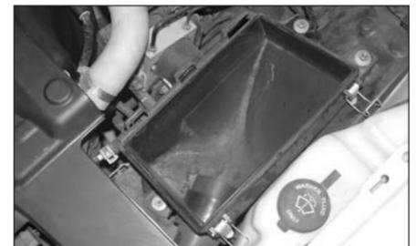
8. Remove the two 11mm bolts that retain the airbox bottom to vehicle.
