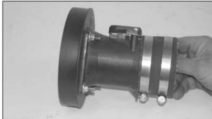
23. Install the silicone hose (08690) onto the mass air sensor with provided hose clamps as shown.
