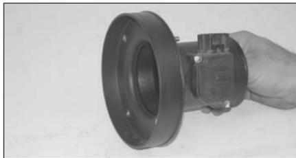
22. Assemble the filter adaptor onto the mass air sensor with the provided hardware as shown.
