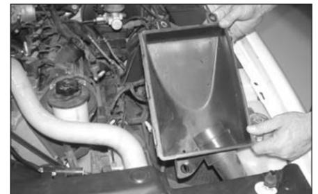
9. Remove airbox bottom from vehicle as shown.
