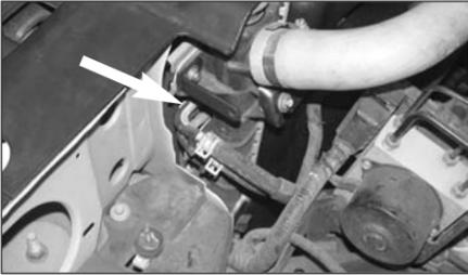
11. Install the provided bracket (07879) onto radiator with the provided hardware.
