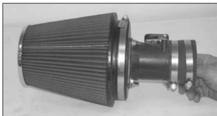
24. Install the filtercharger onto the mass air assembly as shown.
