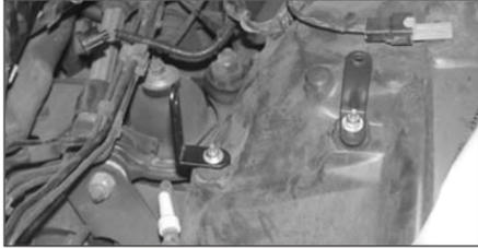
12. Install the two provided bracket onto the factory rubber mounted studs with the provided hardware.
