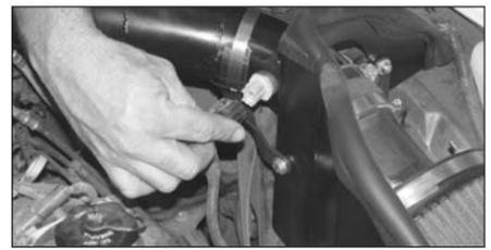
27. On vehicles with external temp sensor, install the temp sensor onto the intake tube then re-connect the electrical connection.
