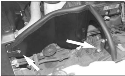
14. Install the heat shield into vehicle and attach to the two outer brackets.
