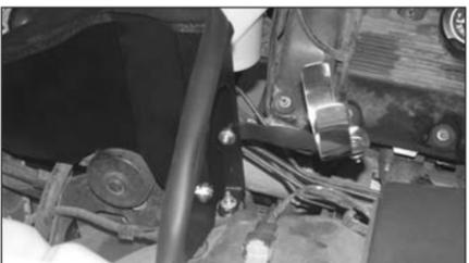
16. Install the saddle bracket assembly onto the heat shield as shown.
