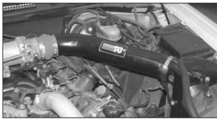
19. Install the K&N intake onto the throttle body and line it up with saddle bracket assembly.
