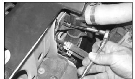
10. Remove the 8mm bolt that retains the radiator fan shroud to radiator.
