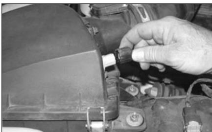
4. Disconnect the temp sensor electrical connection. **Note:** Not all vehicles come with external temp sensors.
