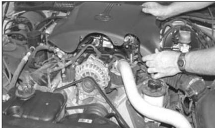
2. Loosen and remove the bolt that retains the engine cover to the engine with a 1/4 extension, then remove engine cover.
