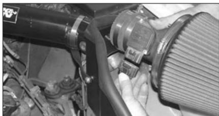
25. Reconnect the mass air sensor electrical connection as shown.
