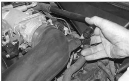
5. Disconnect the crank case vent and ideal air hoses as shown.
