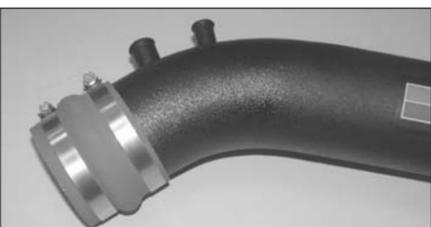
18. Install the provided silicone hump hose (087121) onto the K&N intake tube with the provided hose clamps.
