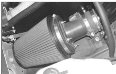
26. Install the mass air assembly onto the intake tube and adjust for best fit before tightening hose clamps.
