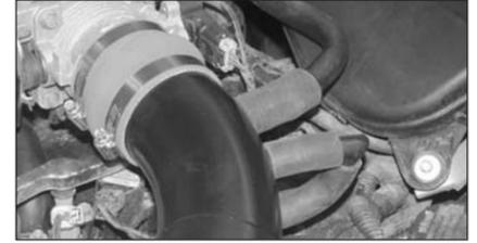
28. Reconnect the crank case vent and ideal air hose onto the new intake tube with the provided silicone hoses as shown.
