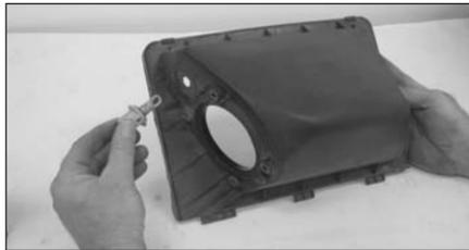
21. On vehicles that come equipped with an external temp sensor, twist counter clockwise to remove from airbox lid.
